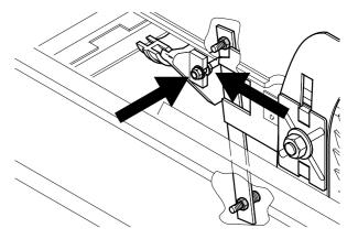
The swivel segments' setting nuts must not be tightened during operation of the saw, as this would create mechanical twisting and warping.
